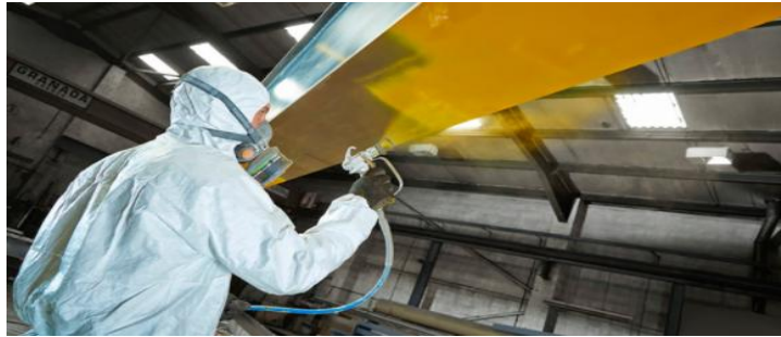
Figure 5. The spray gun coating
